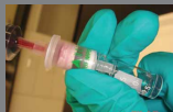
b. Pass red wine extract through the mini-cartridge slowly, collect 0.5 mL cleaned extract
