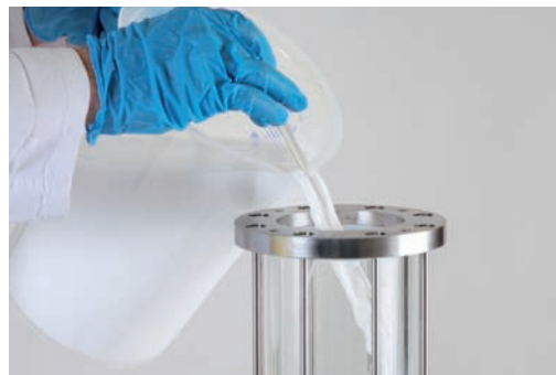
FIGURE 8 Pouring the resin
