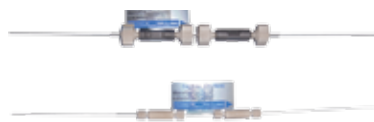
MonoCap C18 Trap Column with Hardware (Top Image: 1/16" End-fittings, Bottom Image: 1/32" End-fittings)
