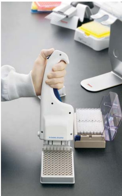
Thermo Scientific decapper caps and decaps 8 tubes at a time
