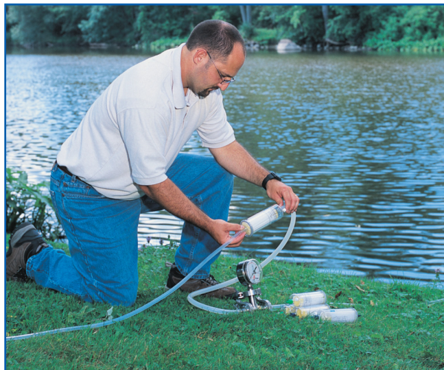
Envirochek HV sampling capsules set the standards for Cryptosporidium and Giardia testing.
